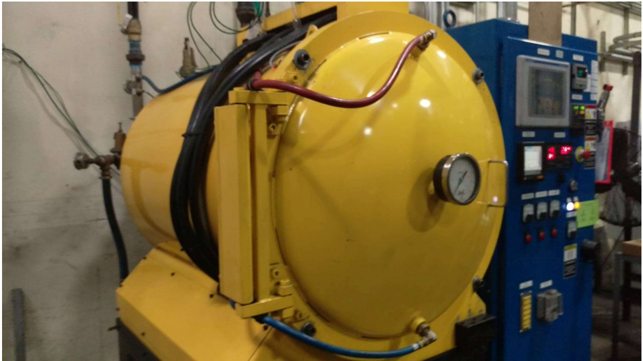
Figure 50. Vacuum Annealing oven used by Stack Metallurgical Co.
