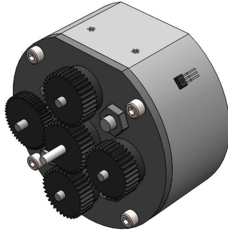
Figure 21 Eight rod circular Halbach activation prototype including external hall sensor
