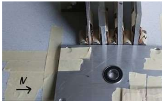
Figure 15. Jig to determine polarization direction for all eight magnets. In the jig, each magnet aligned its south pole with a corresponding magnets north pole. From there, the polarization directions can be easily marked on the face of each magnet.
