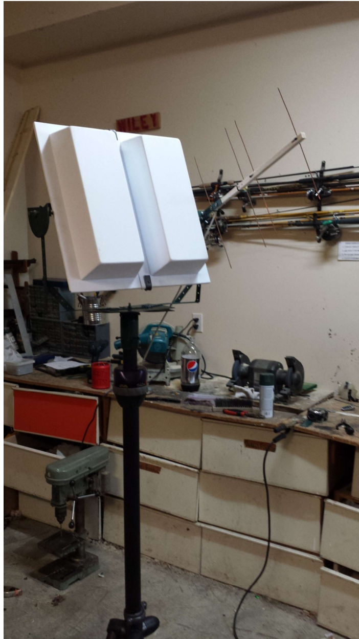
Finished manual antenna tracker
