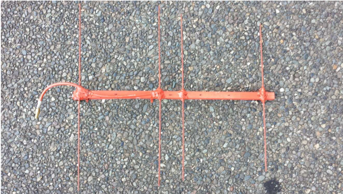
9 dBi four element Yagi antenna
