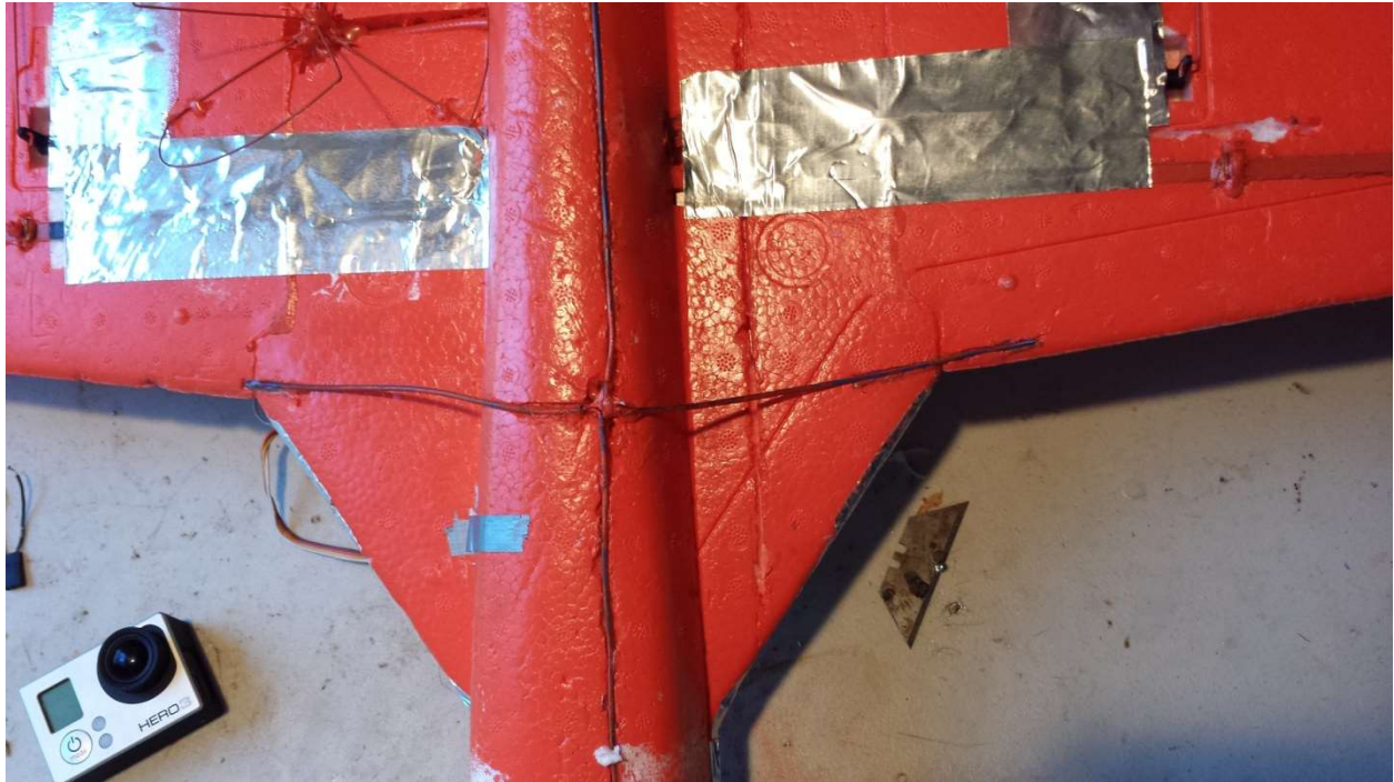
Turnstile antenna mounted on the glider
