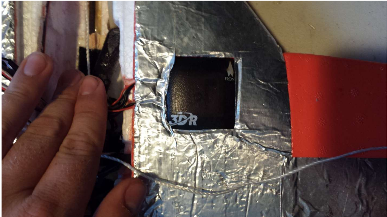
APM GPS mounted in the glider
