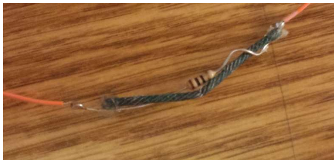
10 \Omega 1/4w resistor and fuse cutoff
