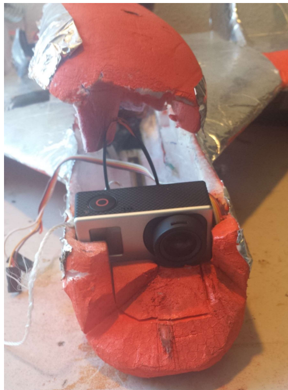
GoPro mounted in glider with video out cable
