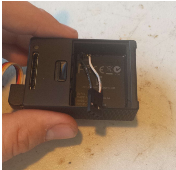
GoPro mounted in glider with video out cable
